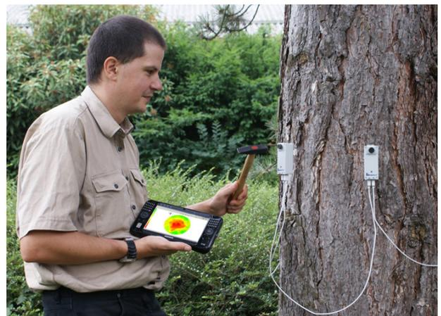
ARBOTOM 应力波断层成像仪
